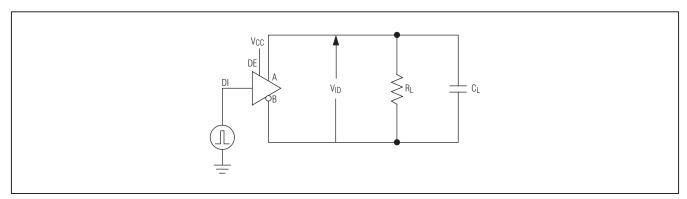
Figure 3. Driver Timing Test Circuit
