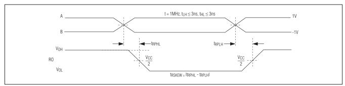
Figure 9. Receiver Propagation Delays
