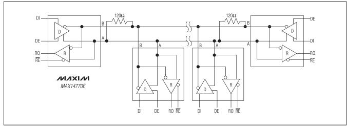
Figure 12. Typical Half-Duplex RS-485 Network
