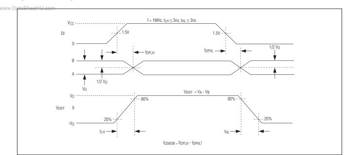
Figure 4. Driver Propagation Delays
