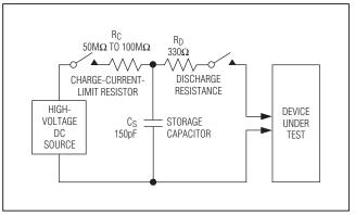
Figure 15. IEC61000-4-2 ESD Test Model
