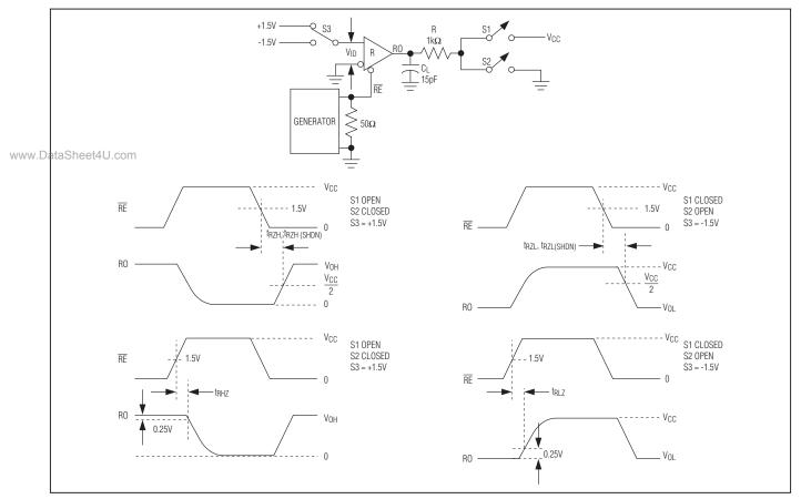
Figure 10. Receiver Enable and Disable Times
