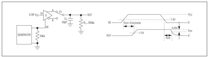
Figure 6. Driver Enable and Disable Times
