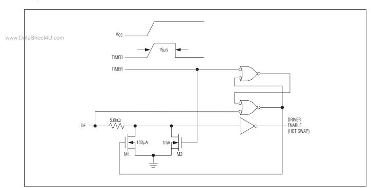
Figure 11. Simplified Structure of the Driver Enable Pin (DE)
