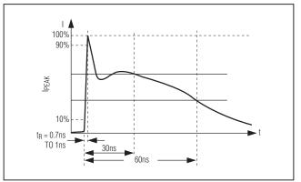
Figure 16. IEC61000-4-2 ESD Generator Current Waveform
