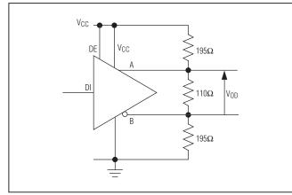
Figure 1. Driver DC Test Load
